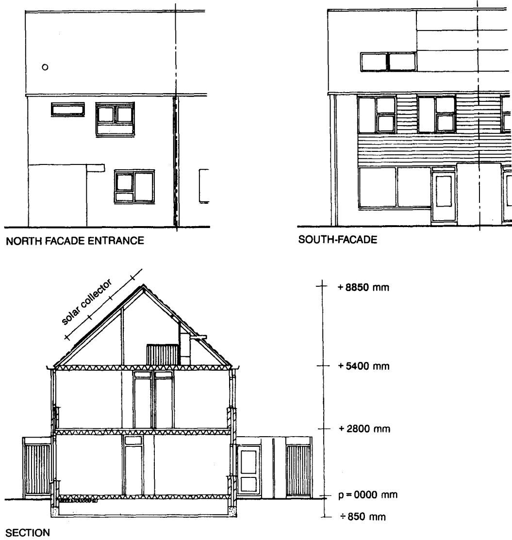
Figure 3: facades and sections
