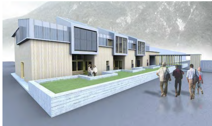
Fig 4.1315: Rendering of an elementary school made of wooden prefabricated elements, including the BIPV prototype on the left. [re-arrangement L. Maturi from rendering Studio Arch. Frate]
