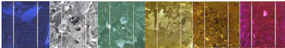
Fig 3.5: Multicrystalline silicon wafers; first the blue antireflective standard colour with the best efficiency, the second is the original wafer without reflective layer, then cells with other colours that have different anti-reflective layers, © Sunways
