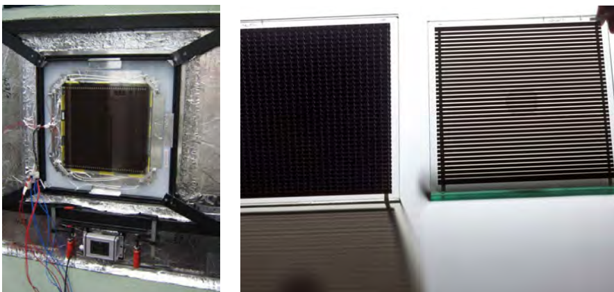
Fig 4.412: Fully functional BIPV prototype mounted in the test rig at Fraunhofer ISE premises [4.9].
