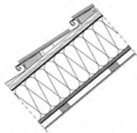
Design structure of QUICKSTEP RHEINZINK® Stepped Roof
