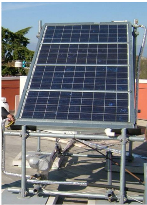
Figure 8: Testing of the MSS Multi solar PV/T collector for electricity, hot air and hot water.
