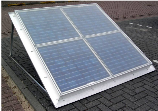
Figure 2: The PVTWIN PV/T collector tested in the project. [8]
