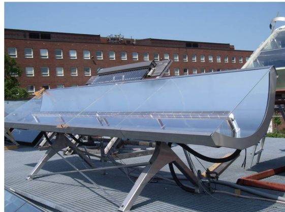
Figure 5: Testing of Solar 8 concentrating PV/T collector for electricity and hot water. [7]
