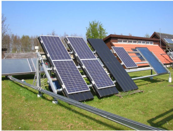
Figure 7: Testing of the SolarWall PV/T collector for electricity and hot air together with a standard solar thermal collector and PV module as references. [9]
