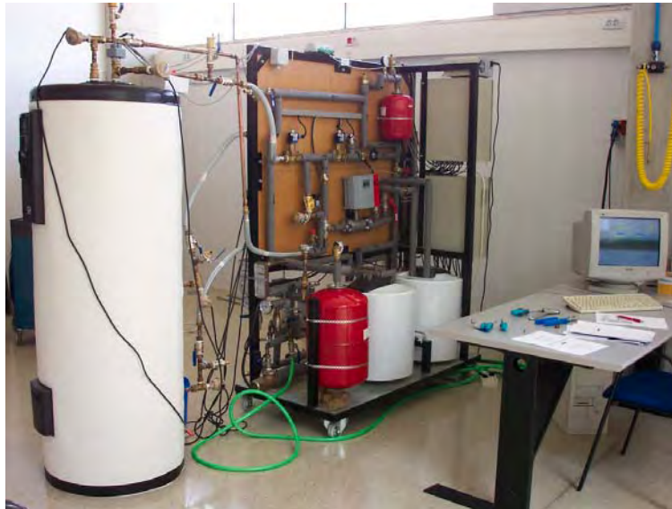
Figure 2-4 Test ring installation and commercial tank used in the experiments.
