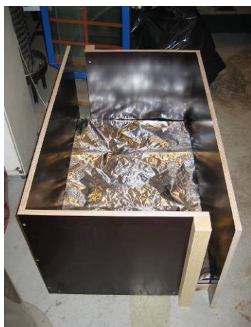
Fig. 2.1.5 Plastic foil bag in plywood box before filling with melted salt solution.
