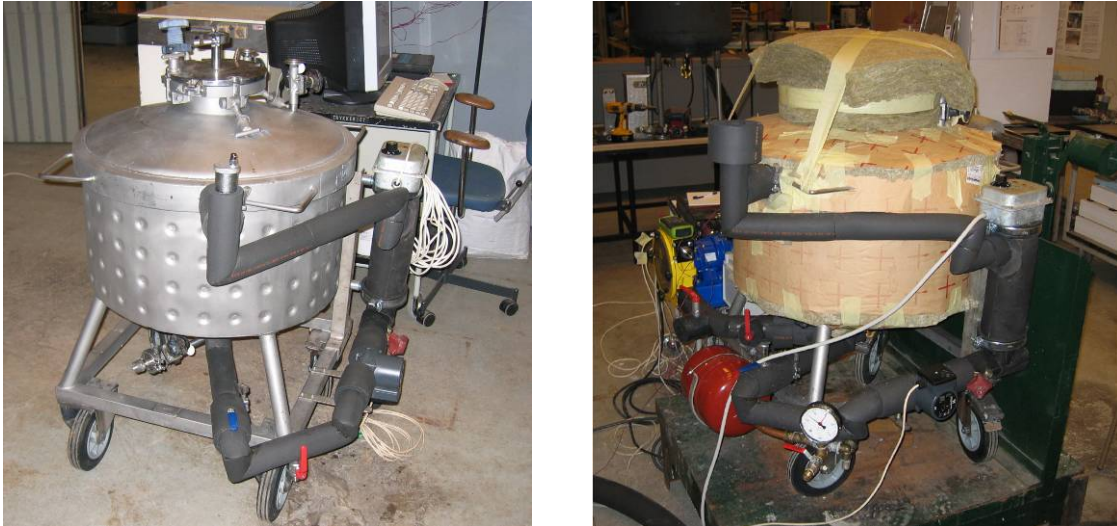
Figure 2.1.3 Left: Stainless steel mantle tank with the water heating loop connected Right: Insulated mantle tank with both water heating loop and salt loop connected. The tube pump can be seen in the back to the left (yellow and blue).
