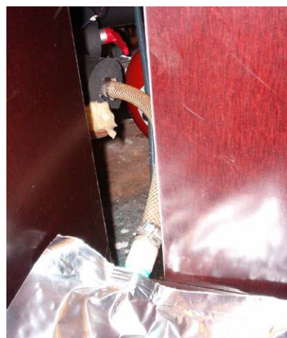
Fig. 2.1.6 Filling of plastic foil bag from the melting tank.
