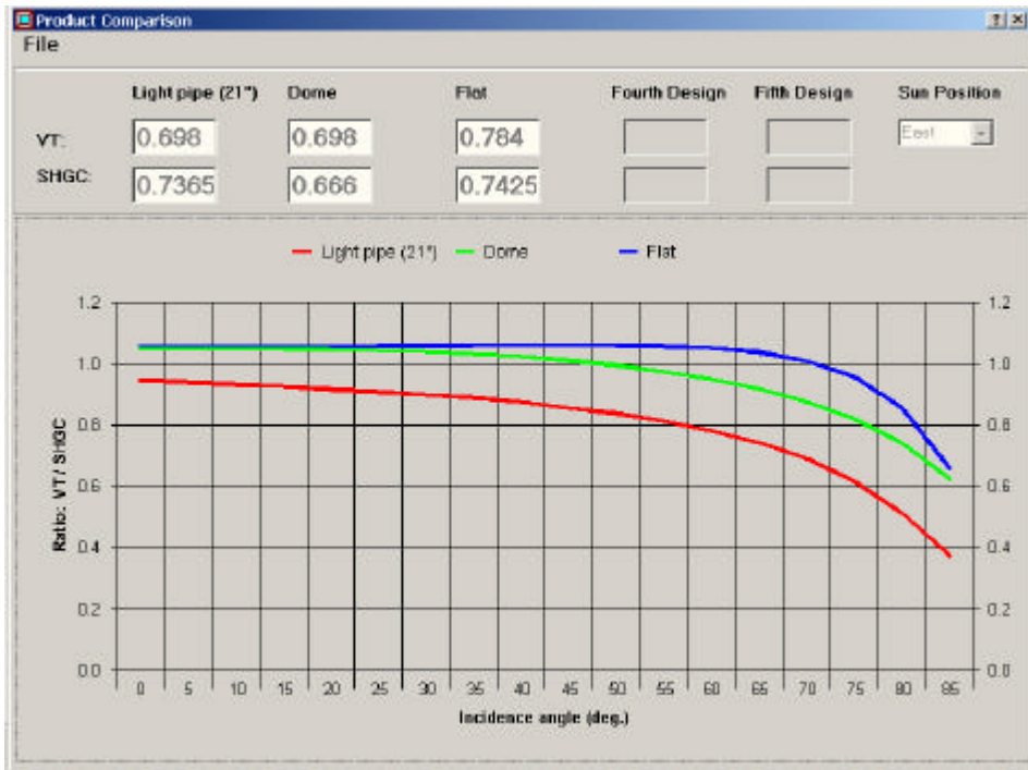
Fig. 4: Comparing skylight products based on the visible transmittance (VT) and solar heat gain coefficient (SHGC): double clear flat skylight, double clear hemispheric dome, and light pipe (21" diameter and 4' length). Domes offer an additional feature of admitting more solar heat gains at low sun altitudes (typical winter days) compared to similar flat skylights.
