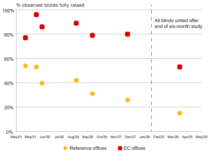
Figure 4. Percentage of Venetian blinds in fully raised position in reference and EC test offices before and after the six-month monitored period. After December, any remaining blinds were untied in the EC test offices.
