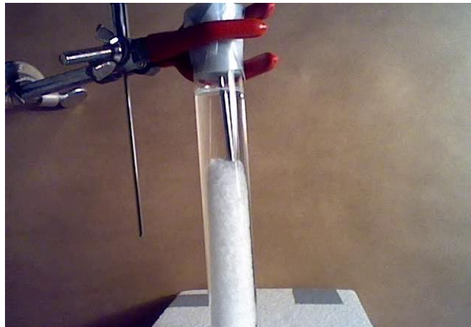
Figure 26: Phase Separation during Melting of Octadecane
