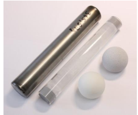
Figure 25: Macroscopic encapsulated PCM for mobile latent thermal energy storage of University of Bayreuth
