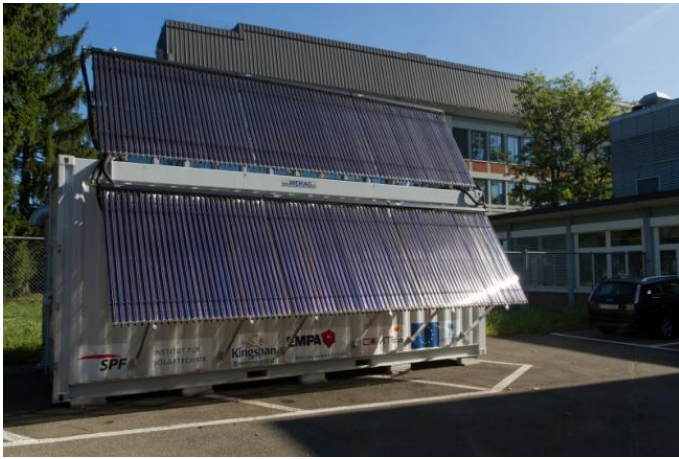
Figure 3: Picture of the demonstrator container from the outside with the vacuum tube collector field.
