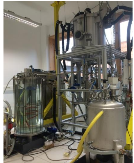
Figure 7: Picture of the PROSSIS2 prototype: in front, the water storage tank, in glass: the solution storage tank, above: the reactor
