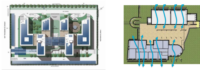
Fig. 2. Green Office and EnerPos building: the width is reduced to use the natural resources (sun, wind...)
