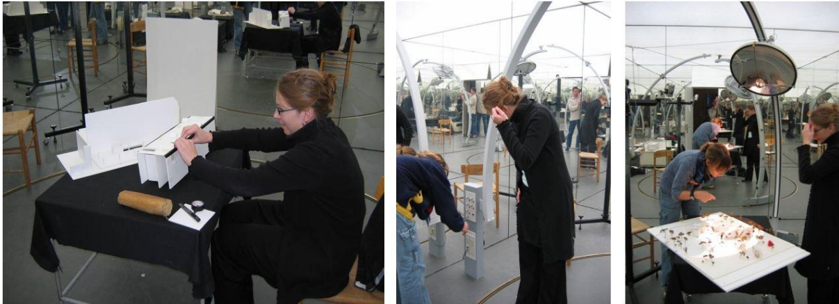
Figure 7: Mirror-box sky and sun simulator at the Royal Academy of Fine Arts School of Architecture in Copenhagen (Photography: Werner Osterhaus).
