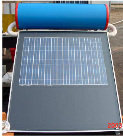
PV/Thermal prototype by with PV on part of the absorber [4].
