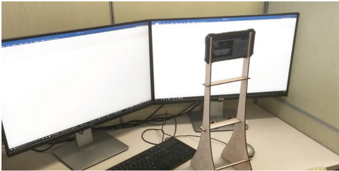
Fig. 4. Calibrated mobile phone device with a micro fish-eye lens to capture HDR images at occupant workstations.
