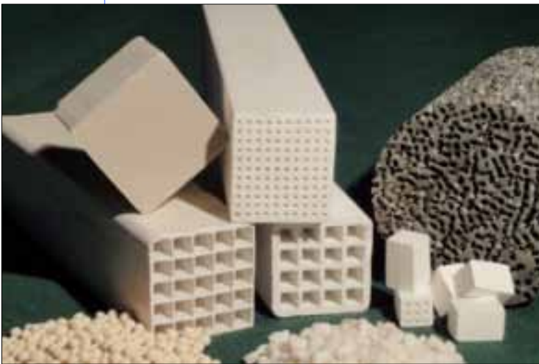
▲ Figure 1. Different composites investigated at ITW: salt/zeolite composites (bottom left), compacted salt granules (bottom right), salt in honeycomb structure with different channel geometries (top left), aluminium foam impregnated with salt (top right).
