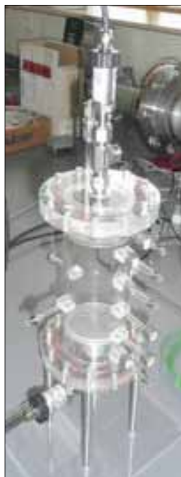
▲ Figure 2. Small experimental reactors to determine the hydration/dehydration characteristics of salt hydrate composites at ECN.
